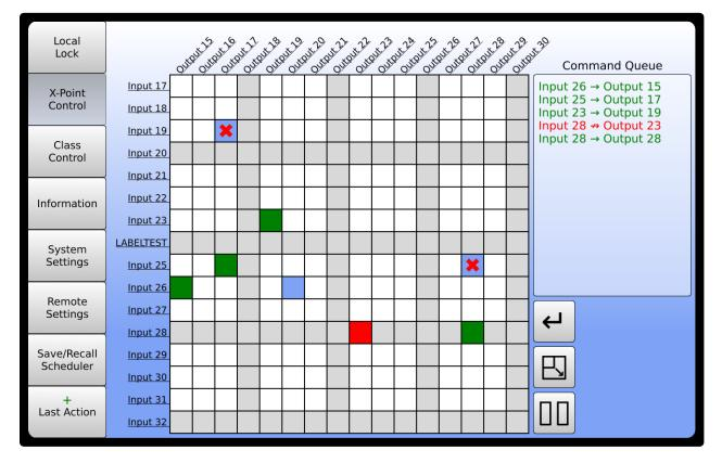
Simply tap the crosspoints you wish to connect (crosspoint will turn green) or disconnect (crosspoint will turn red) and watch as each command populates the Command Queue. Note that outputs that are already connected to a different input will show a red X indicating that the Auto-Interlock feature will disconnect that crosspoint and connect the new crosspoint (see output 19 in the example above).
