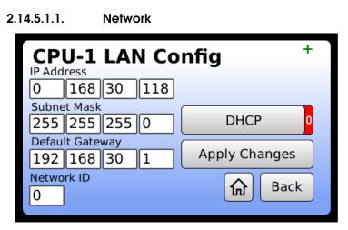
IP Address: If a static IP address is to be used, enter it here. Otherwise a DHCP address will be used.
