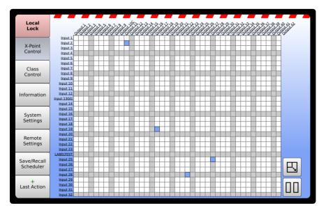
Once the front panel is locked, it must be unlocked before regaining access. Note that remote control access is always available regardless of the status of the lock screen.
