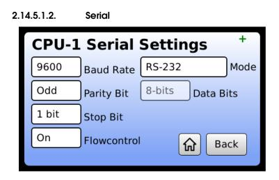
The serial settings menu allows you to configure the serial port to match the serial settings of your host. By pressing any of the available settings, a drop down menu will be activated. Use your finger to scroll through and select the appropriate settings for your environment. Available options are:
