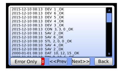
The Error Only button is a Boolean toggle that is either ON (green / I) or OFF (red / 0). By toggling this function ON, you can filter out all events except for those that resulted in an error:
